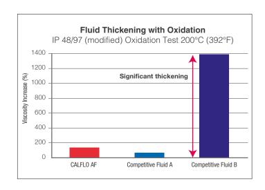
CALFLO AF demonstrates significantly better resistance to viscosity increase versus competitive fluid in a severe oxidation test conducted at an independent industry laboratory.
