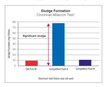
Even at mild 135°C (275°F) temperature conditions, CALFLO AF provides stronger resistance to sludge formation than other competitive fluids.
