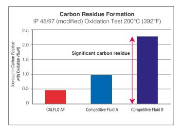
CALFLO AF demonstrates significantly better resistance to carbon residue formation in severe oxidation testing conducted at an independent industry laboratory.
